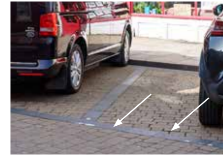
Parking Bays - Black basalt setts
