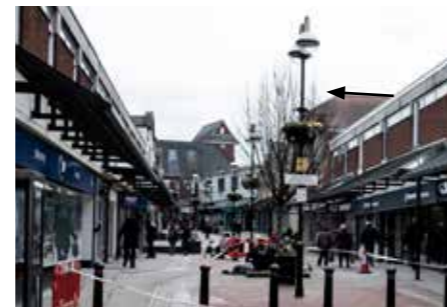
Lighting - Contemporary 6m column lighting with hanging baskets, gold trim and banner mountings
