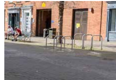
Cycle racks - Stainless steel Sheffield hoops
